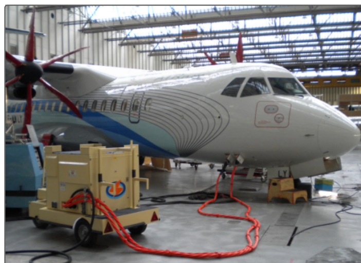
'SFC Combo' 400Hz + 28VDC GPU on all-weather trailer
