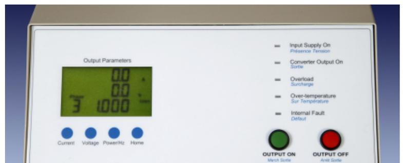
The comprehensive digital display shows output voltage, current, frequency, power and power factor.
